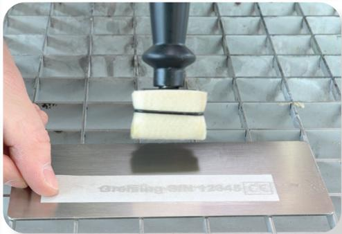
Individual marking patterns are made on customers requirement. Due to the silkscreen method the patterns can be reused up to 500 times.
